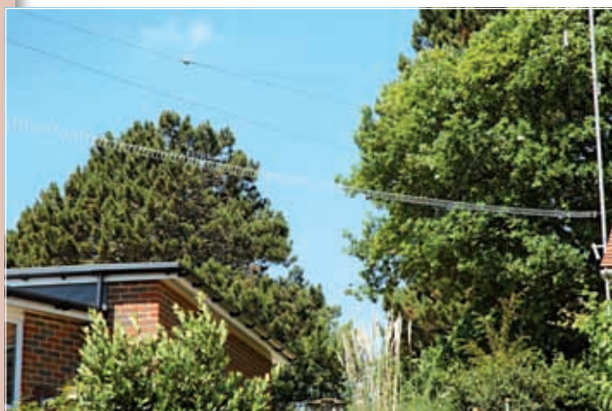
The Slinky antenna running down the garden at John's QTH.
